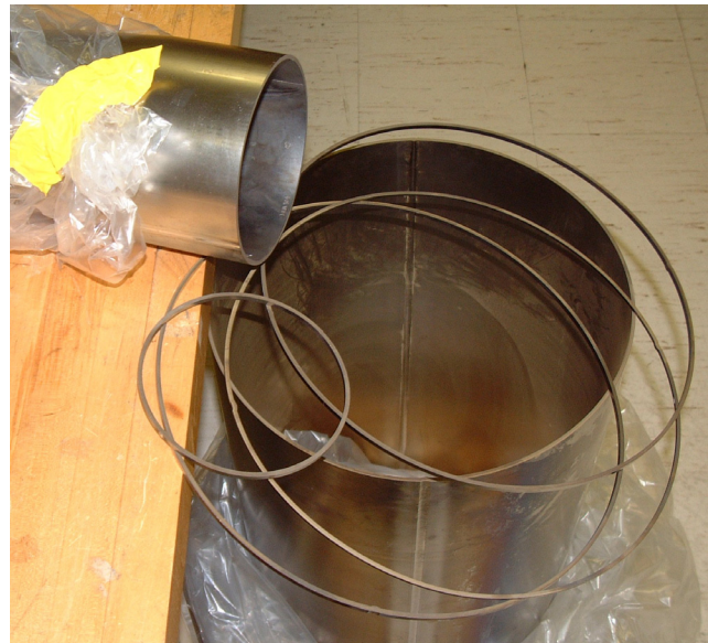
Fig. III-8. Cavity assembly clamped together for frequency measurement (left). Cavity housing and center conductor together with rings of material sliced off using wire EDM for frequency adjustment (right).
