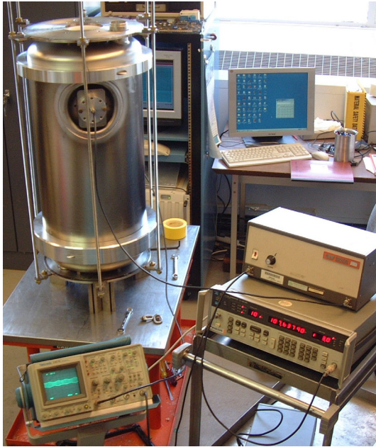
Fig. III-8. Cavity assembly clamped together for frequency measurement (left). Cavity housing and center conductor together with rings of material sliced off using wire EDM for frequency adjustment (right).
