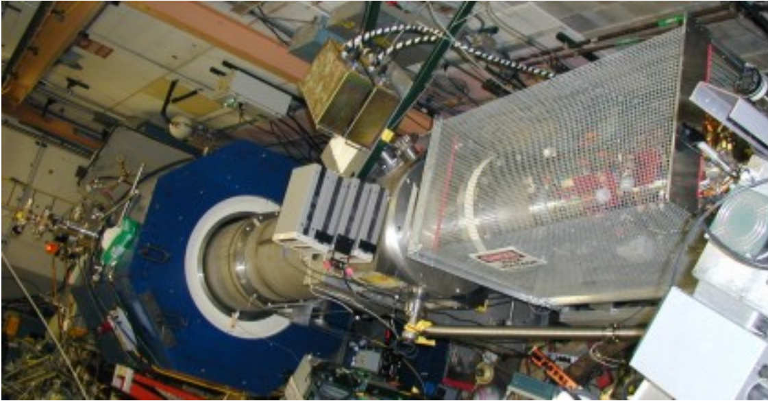
Fig. III-59. Aerial view of the large gas catcher inside its high-voltage shielding cage (on the right) in location at the end of the new beamline built to reproduce the ion properties expected after the final degrader in a RIA-type fragment separator. The main optical element in that beamline is a 65 cm bore superconducting solenoid shown in blue at the left of the picture.
