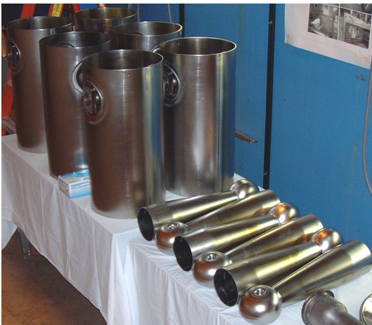
Fig. III-7. Housing/re-entrant nose subassemblies together with center conductor subassemblies for six quarter-wave cavities (left). Center conductor and upper toroid subassemblies are fixtured in vacuum chamber for electron beam welding (right).
